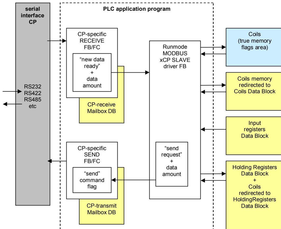
Note: The data is read, checked, transferred and response prepared within the same PLC scan.
